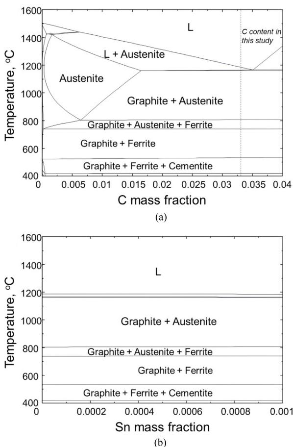
Fig. 8 Phase diagrams plotted for temperature versus (a) carbon mass fraction and (b) Sn mass fraction calculated by FactSage 8.2. The contents of Si and Mn are fixed at 2.1 and 0.7 mass%, respectively, in Fig. 7(a). The contents of C, Si, and Mn are fixed at 3.3, 2.1, and 0.7 mass%, respectively, in Fig. 7(b)
