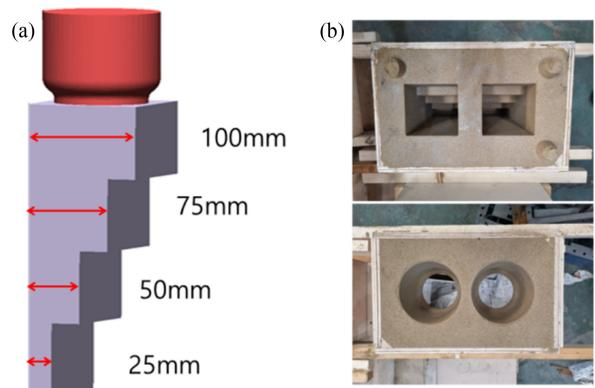
Fig. 1 (a) Geometry and (b) Actual images with pouring cup and riser (lower image) of step casting mold used in this study
