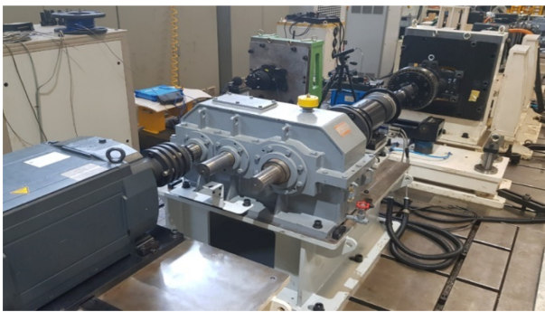
Fig. 16 Test equipment set-up for gearbox
