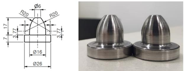
Fig. 3 Dimension and shape of electrode
