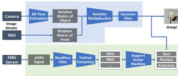
Fig. 5 Flow chart of the control procedure
