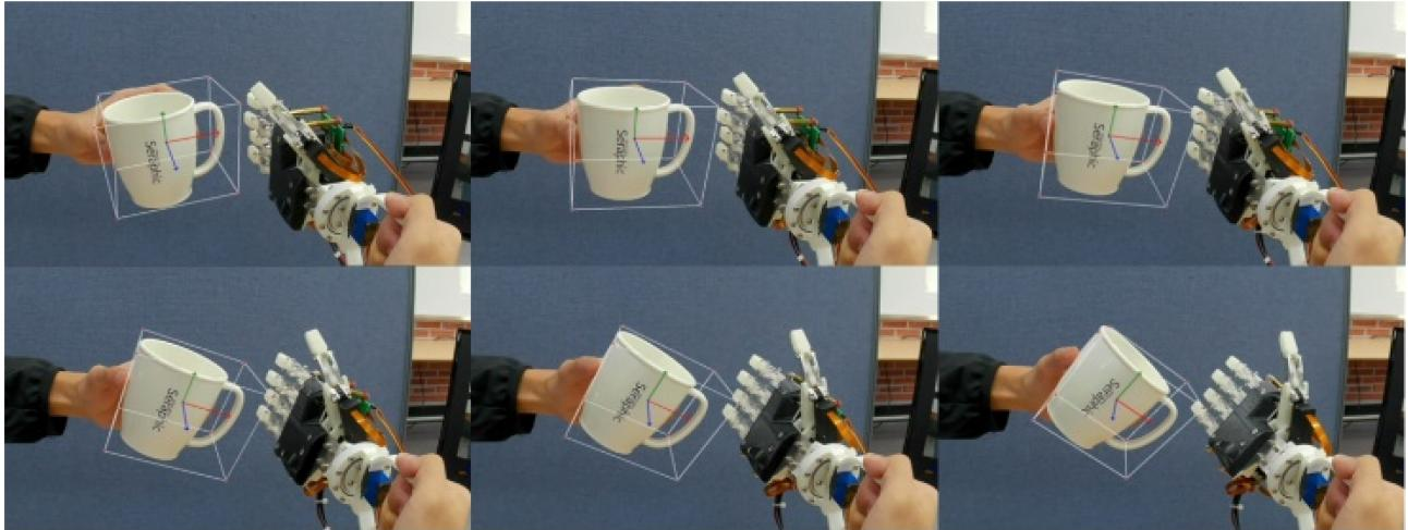
Fig. 8 Demonstration of the wrist control of the prosthetic hand
