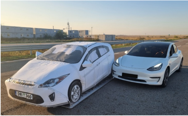
Fig. 4 Guided vehicle target robot test
