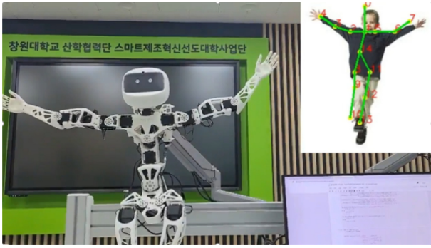
Fig. 6 Data on joint points extracted from photos using openpose applied to actual robot
