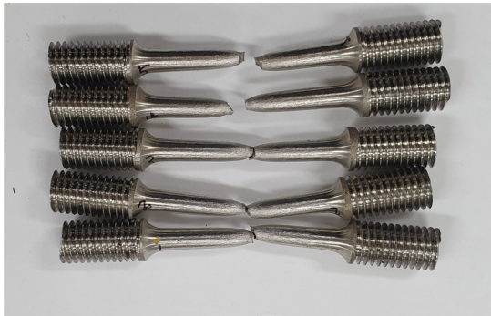
(b) After tensile test specimens (Z-direction)
