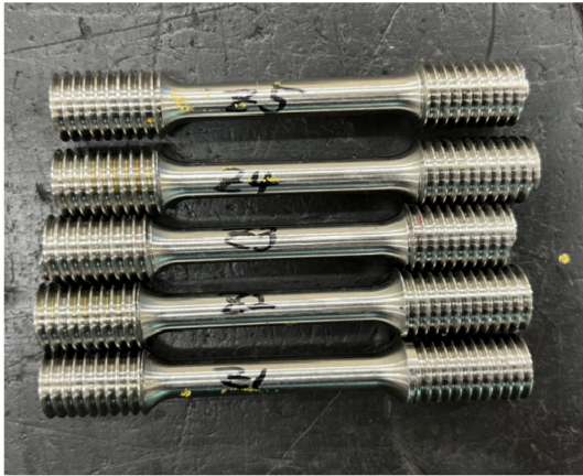
(a) Before tensile test specimens (Z-direction)
