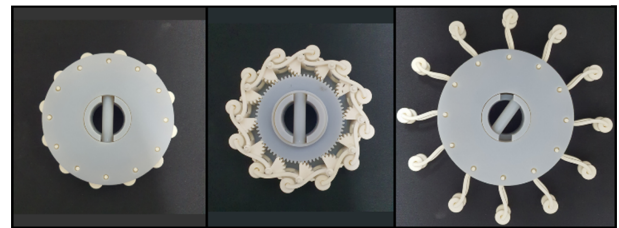
Fig. 13 Diameter-expanding catheter reel 3D printer output
