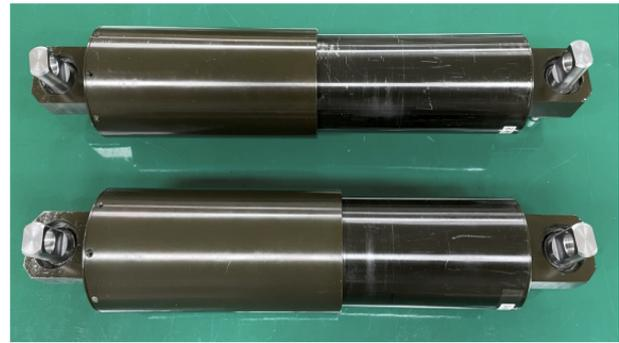
Fig. 2 Test damper used in the field test
