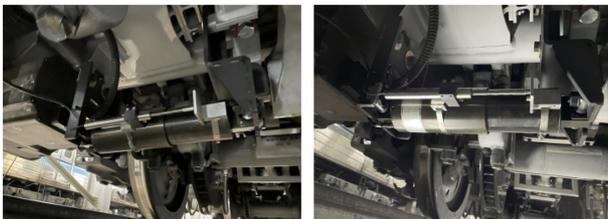
(a) Normal damper (b) Fault damper
