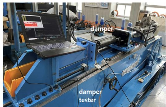
Fig. 6 Damper force calibration test
