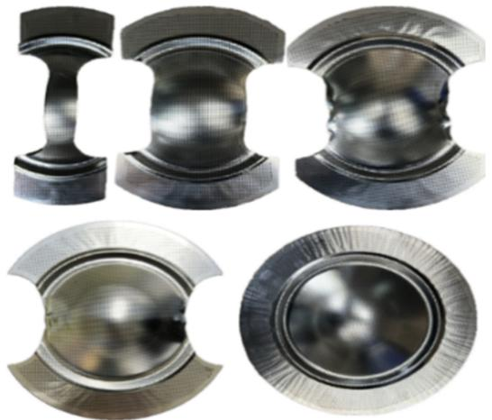
Fig. 6 Specimens of Nakajima test
