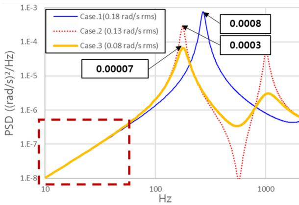
Fig. 9 Comparison results of angular velocity response analysis at counterweight position
