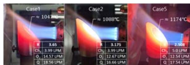
Fig. 10 Photos of flame for the three different burner rig test conditions
