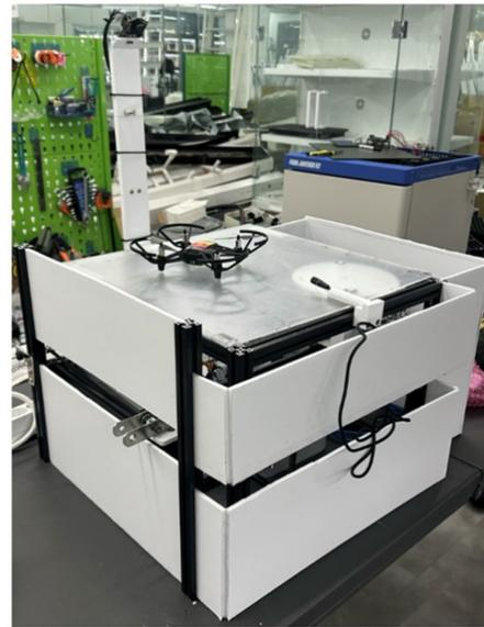
(a) High angle shot image of autonomous drone charging system
