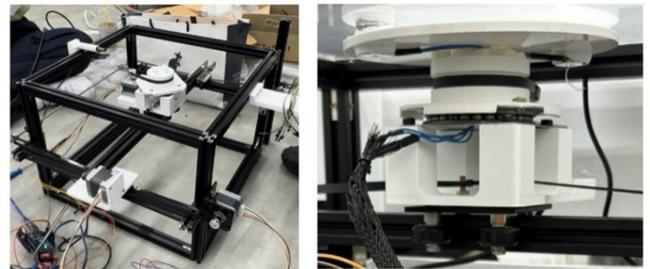
(b) Drone pose alignment manipulator: XY plotter (Left), Rotational plate (Right)
