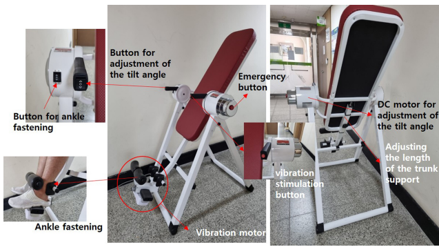
Fig. 1 The vibration stimulation-based inversion table
