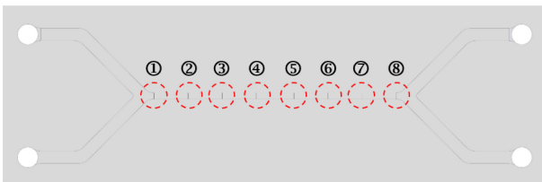
Fig. 7 Microchannel deformation measurement location (Micro)
